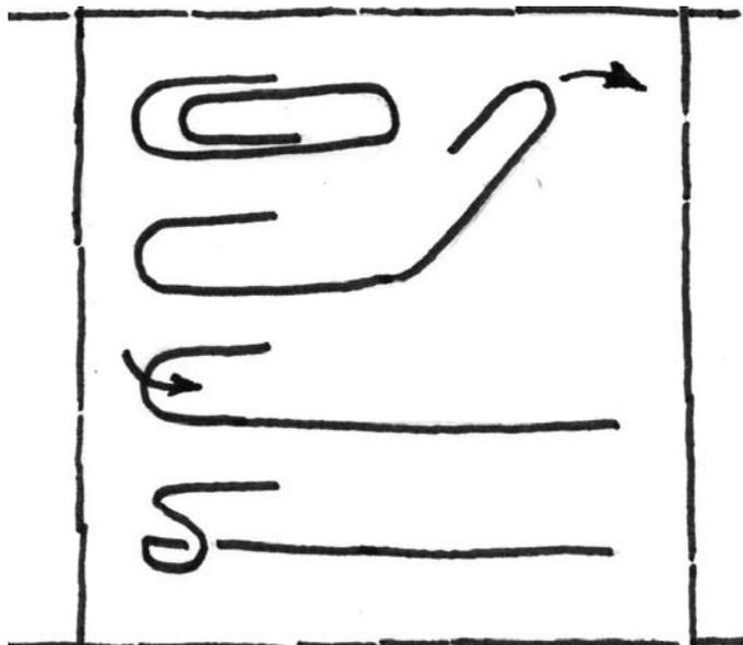
Illustration 1. Lid retractor made from bent paper clip.
